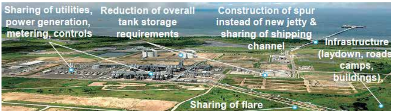
Cost benefits for LNG expansion integration, with material operating and capital expenditure savings.
