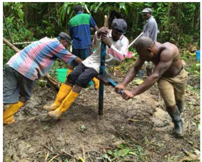
Auger drilling at Orokolo Bay, Gulf Province by Mayur Resources.
