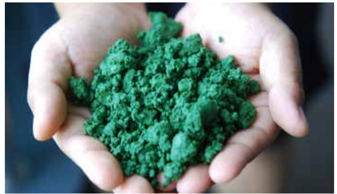
The nickel concentrate that is shipped to buyers. It is usually referred to as mixed hydroxide product (MHP).
