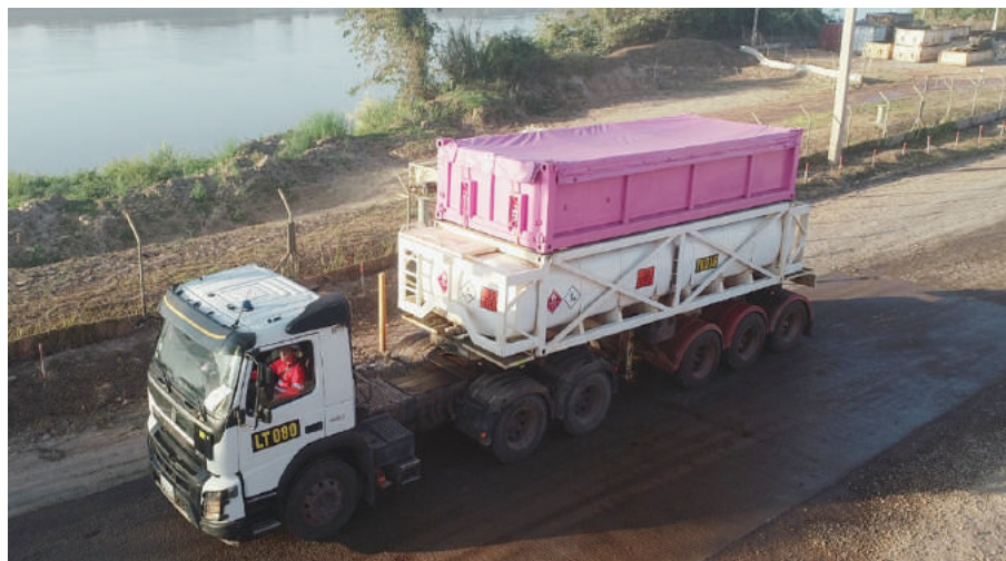
A truck bound for the Phu Kham Copper-Gold Operation loaded with a full fuel tank (bottom) and an empty concentrate container (top). Pic courtesy of PanAust
